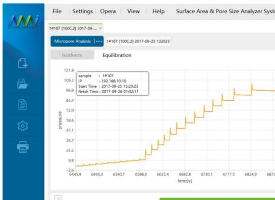
Each adsorption equilibrium process is dynamically displayed on the software interface. Adsorption characteristics of the sample can be easily understood.
